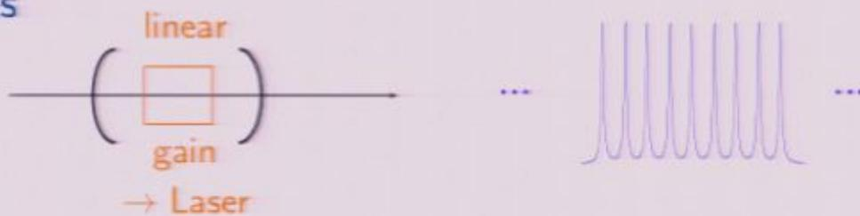
Properly stabilized mode-locked laser = optical frequency comb
