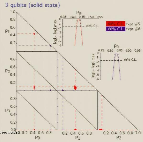
Twirled channel parameters for two time-suspension sequences which differ only in the pulse spacing (10  $\mu$ s vs. 5  $\mu$ s).
