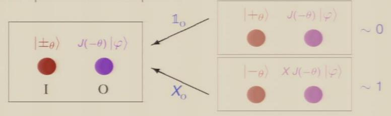
$J(-\theta)$  can be performed using  $|\pm_{\theta}\rangle \propto |0\rangle \pm e^{i\theta} |1\rangle$  measurements
