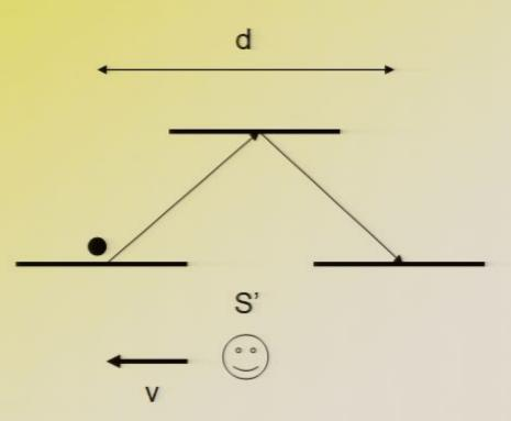
$$\Delta t' = \frac{\text{distance}}{\text{speed}} = \frac{2\sqrt{L^2 + \left(\frac{d}{2}\right)^2}}{c}$$
