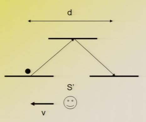
$$\Delta t' = \frac{\text{distance}}{\text{speed}} = \frac{2\sqrt{L^2 + \left(\frac{d}{2}\right)^2}}{c}$$
