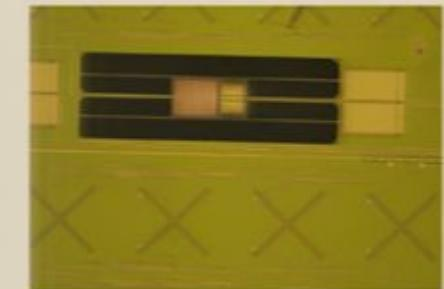
Figure 12: 4-inch-diameter wafer with  $8 \times 8$  spatial pixels (left) and a closeup on a released TES and four antenna pairs at  $50\times$  magnification (right).
