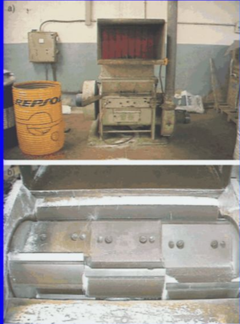
Fig. 1.— a) A photograph of the rotary cutter machine (grinder) used by the patient at the plant at Eurotecno, Barcelona (Spain). b) Detail of the rotary cutter blades.
