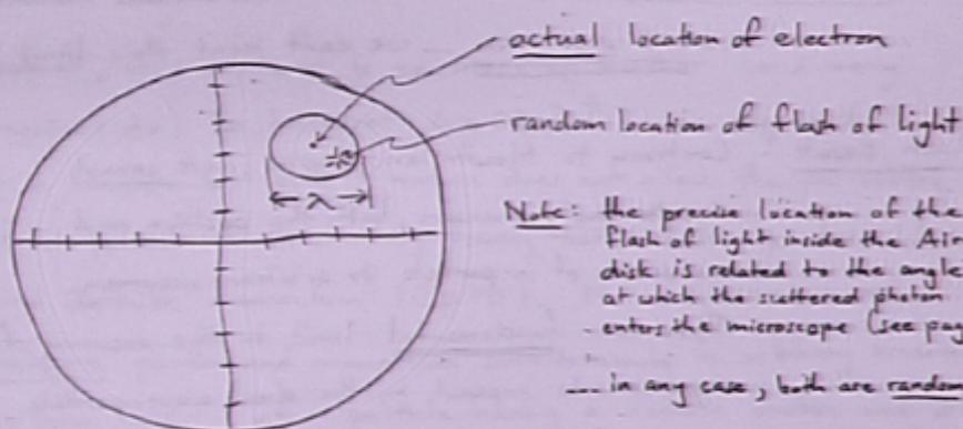
Note: the precise location of the flash of light inside the Airy disk is related to the angle at which the scattered photon enters the microscope (see page 10).
