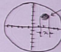
Regardless of the shape and size of the object, we "see" just a fuzzy disk (called an "Airy disk"), whose diameter according to the calibrated grid is about equal to the wavelength of light being used — no details of the object are apparent.
